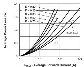
Fig. 4 - Forward Power Loss Characteristics
